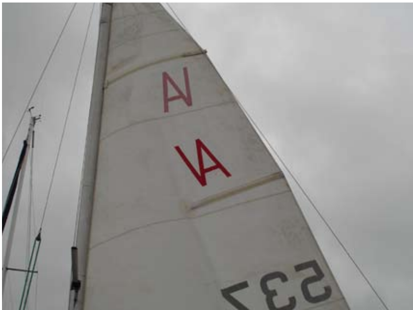
The main was obviously worn out during the last twenty years of use. Rust stains, stretched leeches and a bad shape are the result.
