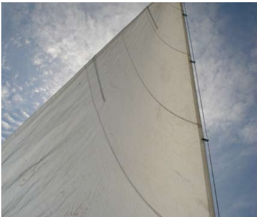
The profile of the jib was distorted along the battens, the leech was loose and the cloth had become way too soft. Rust stains were visual shortcomings.
